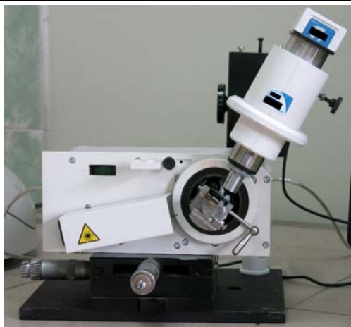
Fig. 1. Experimental setup for visualization of submicron particles by SPR-enhanced total internal reflection microscopy.
